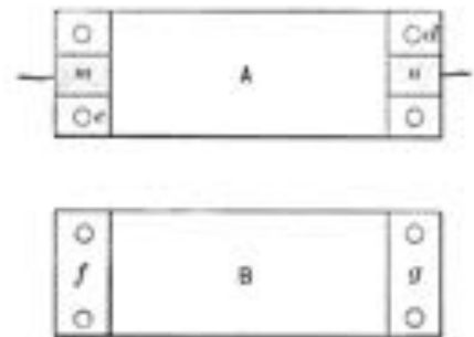
Figure 1: Stone's thin film experiment using silver deposited on glass plates [7].
