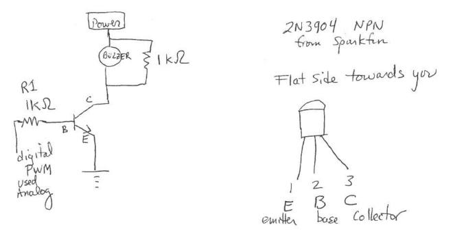
Attach it to power at 5 V, 9 V, 12 V, and run the sketch you used before. Can you hear the difference in loudness? Or put a bench power supply on it and run it up to 30 V.
