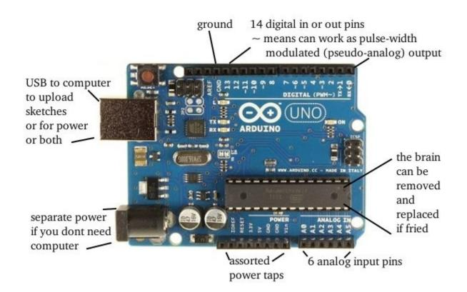
The Arduino gets power either from the USB cable, or from the separate power jack. You don't need both. If you are working with a computer, just use the USB since you'll also use it for communication and uploading code to the Arduino board. Once you have a program "done" and working though, the device could run with power supplied and no connection to the computer.
