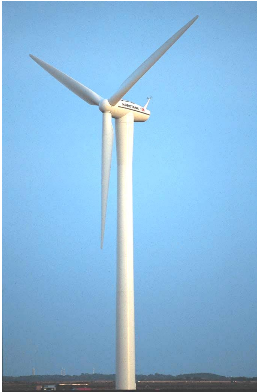
Fig. 1. NEG Micon 1.5 MW wind turbine, 68 m diameter rotor, tubular steel tower. Blades are made of fiberglass. The rotor blades can be turned to optimize power and the entire tower is rotated to face the wind. ([5], "Megawatt-Sized Wind Turbines")
