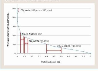
**Figure 2.B2.1** Thermodynamic minimum work per kg of  $\mathrm{CO}_2$  separated from air vs. initial  $\mathrm{CO}_2$  concentration, at 25°C, for the limiting condition that in the end state all of the  $\mathrm{CO}_2$  is separated and pure.
