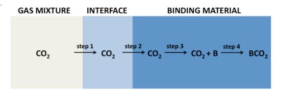
These consecutive steps are linked, where changes in a step later in the chain may impact earlier steps. For example, as CO<sub>2</sub> reacts with a binding site B to form the BCO<sub>2</sub> complex, additional CO<sub>2</sub> may move into the phase containing the binding sites, followed by more CO<sub>3</sub> transitioning through the interface from the gas phase.
