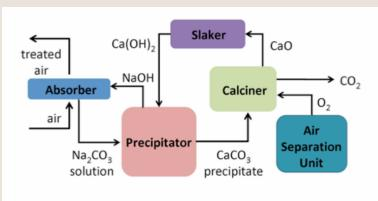
Figure 2.B5.1b. Scheme of a plant for CO<sub>2</sub> capture from air that uses NaOH as the absorber. The pulp and paper industry calls the reactor labeled "precipitator" a "causticizer." In this reactor, calcium carbonate is precipitated and sodium hydroxide (popularly called "caustic soda" as well as "lime") is regenerated.
