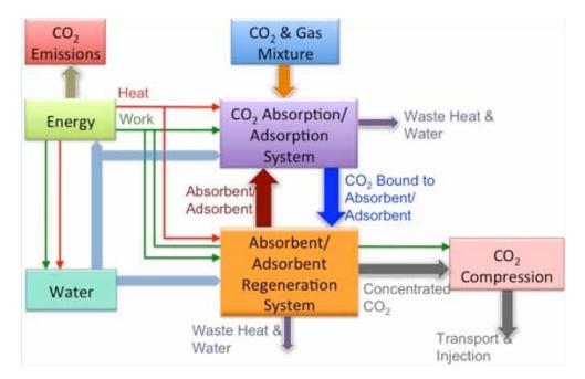
Figure 2.1 A typical system for CO, capture. One key component is a CO<sub>3</sub> absorption/ adsorption system where CO<sub>3</sub> is chemically bound to another molecule, and removed from the gas mixture. The other key component is an adsorbent/absorbent regeneration system where CO, is released in a concentrated form, which is then compressed. These processes require energy (heat and work) and water. Work is in the form of electrical or mechanical power.
