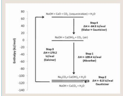
Figure 2.B5.1a. Enthalpy level diagram for CO<sub>2</sub> absorption and regeneration by sodium hydroxide (NaOH). Note that each level has the same set of atoms. In the system studied here, some molecules do not participate in specific physical processes; for example, ideally, NaOH is not transported to the calciner, nor does Ca(OH)<sub>2</sub> participate in the absorption.
