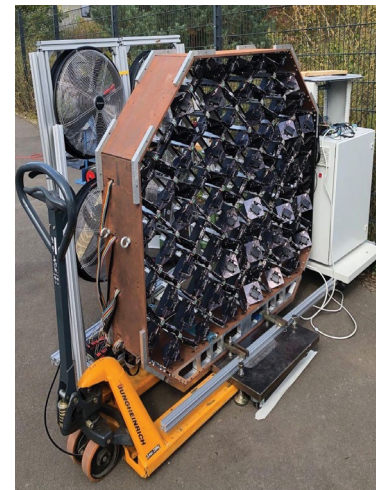
Hejazi and his colleagues manufactured turbulence using four fans behind a grid array with movable flaps. Credit: Bardia Hejazi
