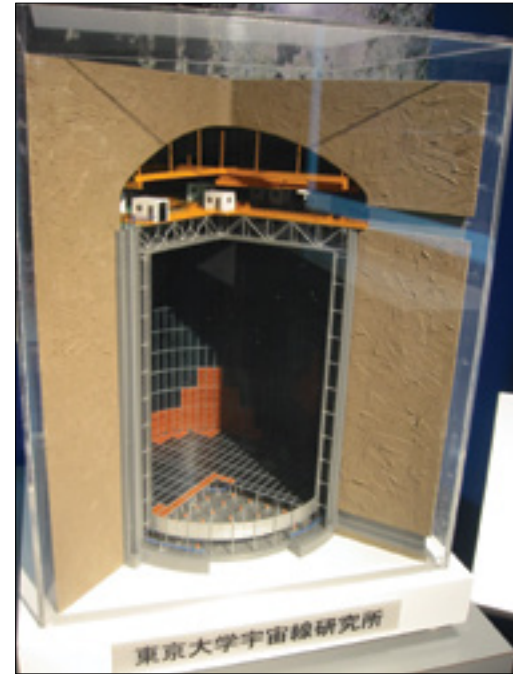
MODEL OF THE KAMIOKANDE DETECTOR
