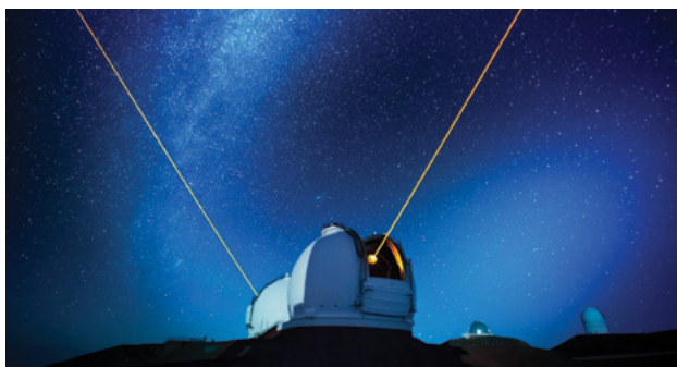
The W. M. Keck Observatory uses a laser (yellow) to create an artificial guide star that allows images to be corrected for atmospheric blurring. Nobel Laureate Andrea Ghez and her team used the facility in her prize-winning research. IMAGE: KECK OBSERVATORY
