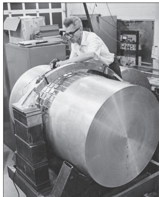
University of Maryland Physics Professor Joseph Weber (1919-2000) with a gravitational wave detector. IMAGE: SPECIAL COLLECTIONS AND UNIVERSITY ARCHIVES, UNIVERSITY OF MARYLAND LIBRARIES
