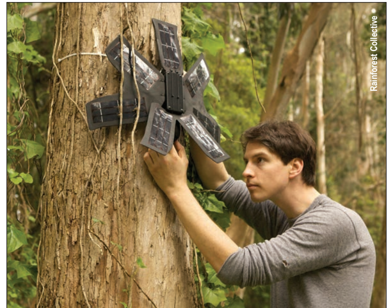
Topher White adjusts a solar array that powers a cellphone being used as a detector of illegal logging.
