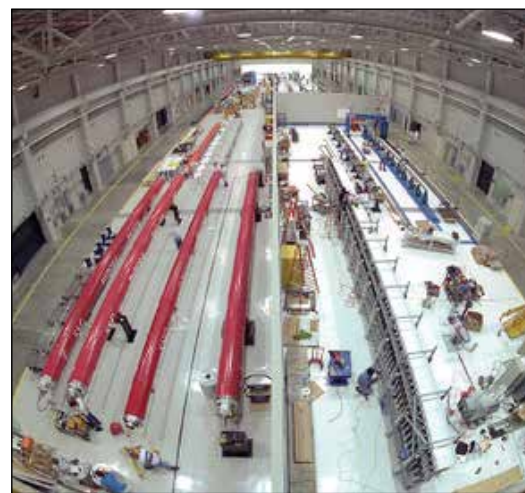
The old interior of the Magnet Development Laboratory where technicians coiled superconducting niobium wires to make powerful magnets.
