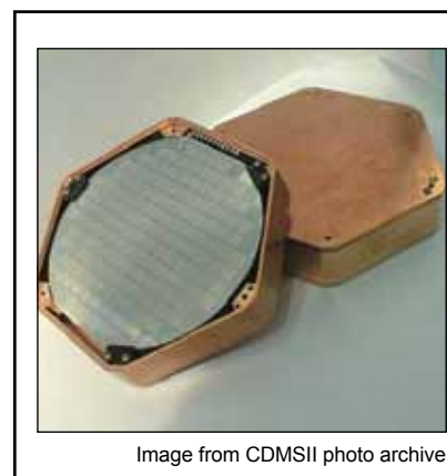
Closeup of a ZIP detector in its mount. A detector of this kind, made of Si, was operated in the 1998 run. The photolithographically-fabricated thin film on the surface is the phonon sensor and represents a significant advance over the detectors used in the 1999 run. Silicon and germanium ZIPs, weighing 100 g and 250 g respectively, will be used in future CDMS II runs at Stanford and in the Soudan mine.
