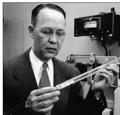
Calvin S. Fuller at work diffusing boron into silicon to create the world's first solar cell
