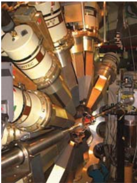
Close-up of Gammasphere, with the G-factor target chamber installed
