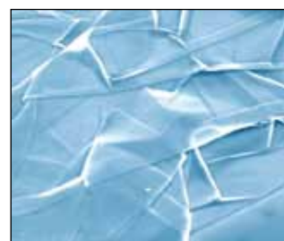
Scanning electron micrograph of a strongly crumpled graphene sheet on a silicon wafer (Foundation of Fundamental Research on Matter, the Netherlands).
