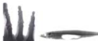
Pictures of a hand and a fish taken with a carbon-nanotube source of x rays. (Courtesy UNC/Applied Technologies)
