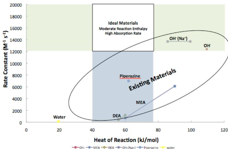
**Figure 3B.1.** Rate constant (liter/mol-sec) vs. absolute value of the reaction enthalpy (kJ/mol) for chemical sorbents.
