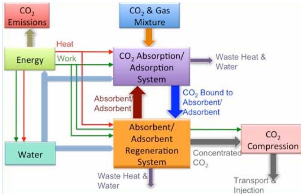
**Figure 2.1** A typical system for CO<sub>2</sub> capture. One key component is a CO<sub>2</sub> absorption/adsorption system where CO<sub>2</sub> is chemically bound to another molecule, and removed from the gas mixture. The other key component is an adsorbent/absorbent regeneration system where CO<sub>2</sub> is released in a concentrated form, which is then compressed. These processes require energy (heat and work) and water. Work is in the form of electrical or mechanical power.
