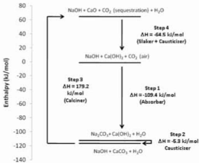
**Figure 2.B5.1a.** Enthalpy level diagram for CO<sub>2</sub> absorption and regeneration by sodium hydroxide (NaOH). Note that each level has the same set of atoms. In the system studied here, some molecules do not participate in specific physical processes; for example, ideally, NaOH is not transported to the calciner, nor does Ca(OH)<sub>2</sub> participate in the absorption.
