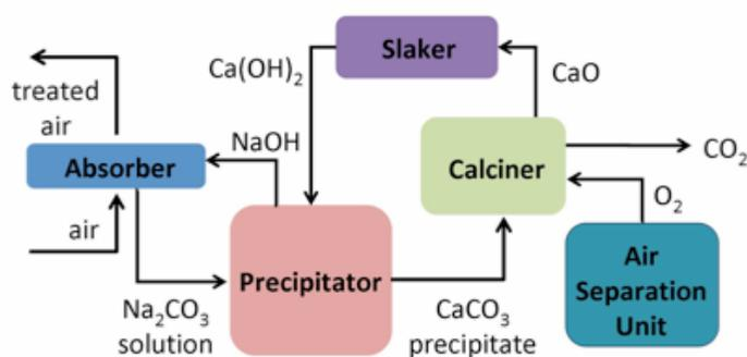
**Figure 2.B5.1b.** Scheme of a plant for CO<sub>2</sub> capture from air that uses NaOH as the absorber. The pulp and paper industry calls the reactor labeled “precipitator” a “causticizer.” In this reactor, calcium carbonate is precipitated and sodium hydroxide (popularly called “caustic soda” as well as “lime”) is regenerated.
