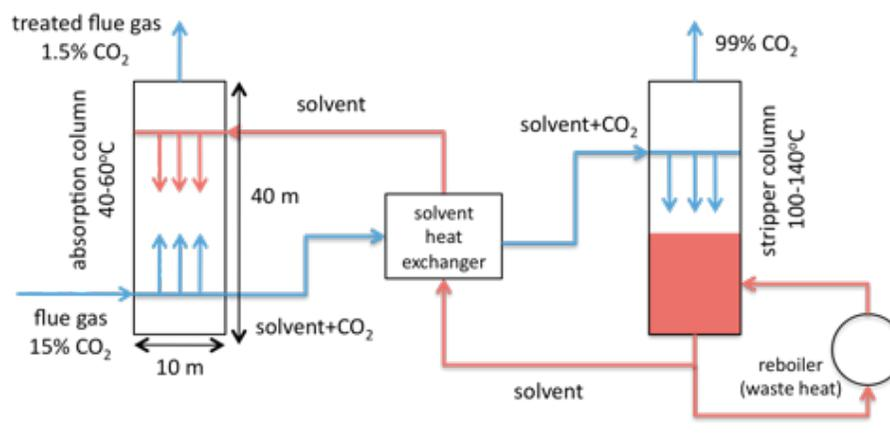
**Figure 2.2** Schematic of a CO<sub>2</sub> absorption system used for post-combustion capture based on the report DOE/NETL-401/110907.
