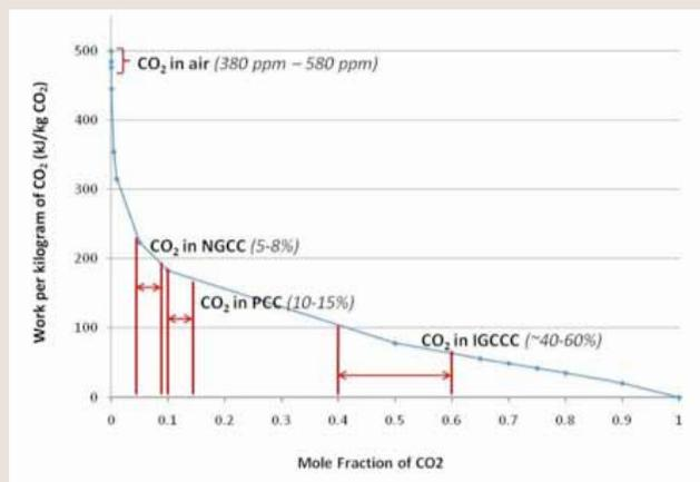
Figure 2.B2.1 Thermodynamic minimum work per kg of CO<sub>2</sub> separated from air vs. initial CO<sub>2</sub> concentration, at 25°C, for the limiting condition that in the end state all of the CO<sub>2</sub> is separated and pure.
