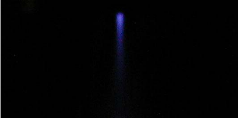
Top Photo: A 20 mA 150 KeV electron beam propagating in air without expanding as a conventional non-vacuum electron beam would.
